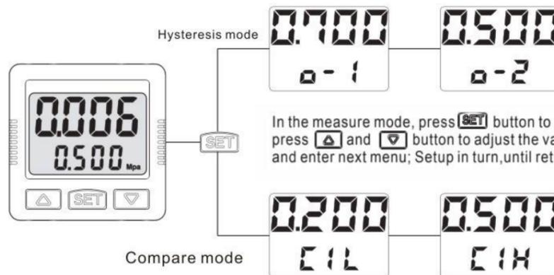
In the measure mode, press **SET** button to enter easy setting mode, press  $\Delta$  and  $\nabla$  button to adjust the value; press **SET** button and enter next menu; Setup in turn, until return to measurement interface.
