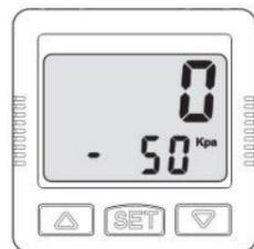
In the measure mode, press  $\Delta$  +  $\nabla$  button at the same time, until display "0", release the button;
