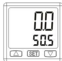
In the measurement mode, press the set key to directly set the switch point value of the current auxiliary display, and support long press to change quickly.
