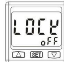
Lock: in measure mode, press + until "LOCK ON" shown;
