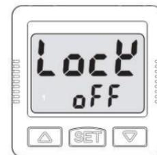
Lock: in the measure mode, press  $\Delta$  + **SET** +  $\nabla$  button at the same time until "LOCK ON" shown, release the buttons;
