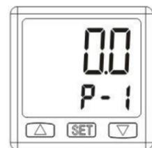
In the measurement mode press the set key to switch the auxiliary display to display the value set by the corresponding switch.
