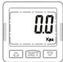
In the measure mode, press + button at the same time, until display "0", release the button;
