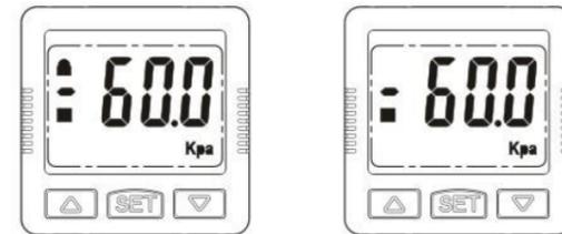
Lock: in the measure mode, press + + button at the same time until "LOCK ON" shown, release the buttons;
