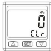
In the measure mode, press button at the same time, until display "o", release the button
