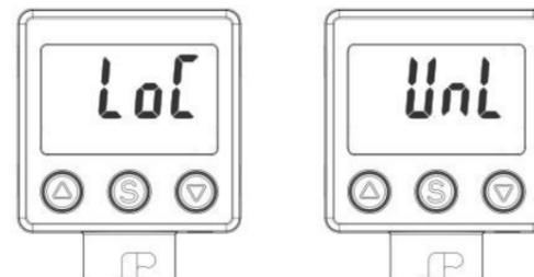
Lock: in the measure mode, press  $\Delta$  +  $\text{S}$  +  $\nabla$  button at the same time until "LoL" shown, release the buttons;
