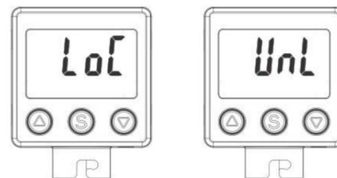
Lock: in the measure mode, press  $\Delta$  +  $\text{S}$  +  $\nabla$  button at the same time until "LOC" shown, release the buttons;
