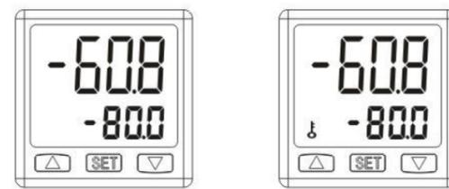
Lock: In the measure mode, press at the same time until "LOCK ON" shown, release the buttons
